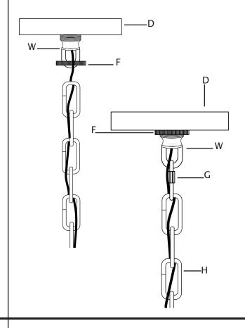
32. Screw recommended bulbs (E12 candelabra bulb type, not included) into sockets. Verify correct bulb wattage marked on socket of fixture. **WARNING:** DO NOT exceed maximum bulb wattage.
