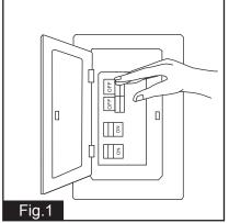
Turn off the electric power at the main fuse or circuit breaker box.
