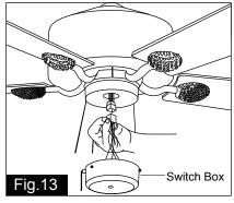
Connect the two terminals respectively from the motor and the switch box.
