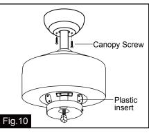
Attach the canopy to the hanger bracket and secure it with canopy screws.
