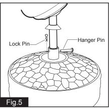
Insert the hanger pin through the holes in the collar and downrod. Insert the lock pin through the hole near the end of the hanger pin until it snaps into its locked position. Finally, tighten downrod screws on the top of the fan motor.
