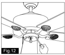
Secure blade brackets to the motor with motor screws and washers.
