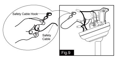
Hang the safety cable into the safety cable hook.
