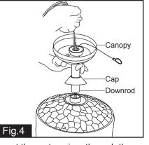
Insert the motor wires through the cap, canopy and downrod.
