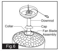
Attach the cap onto the fan blade assembly to cover the collar.
