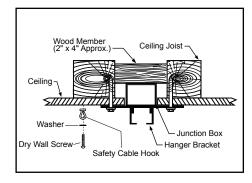
Tighten the hanger bracket to the outlet box with two mounting screws.(Make sure the outlet box is securely installed so that it will be able to support at least the fan weight.) Attach the safety cable hook to the ceiling with the dry wall screw and washer, and make sure the safety cable hook is covered by the fan canopy. WARNING: MOUNT ONLY TO AN OUTLET BOX MARKED "ACCEPTABLE FOR FAN SUPPORT"!
