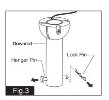
Remove the lock pin from hanger pin and remove the hanger pin from the downrod.
