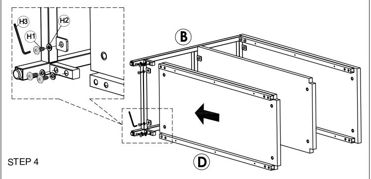
Attach Leg ( B ) to Hole of Table Top ( A ) , Shelf ( C ) and Base ( D ) then secure with the bolts ( H1 ) ,Spring Washers ( H2 ) Tighten the bolts ( H1 ) with provided Allen Key ( H3 )  $\,$
