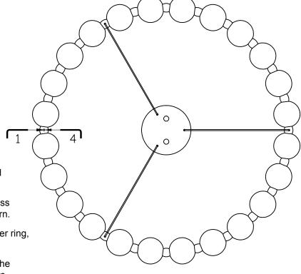
• Remove a screw away from the wire and pull out the aluminum ring connector.
