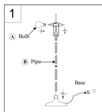
Screw on the bulb (A) make sure this is done with the power off.
