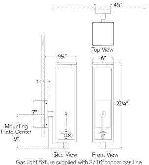
Gas light fixture supplied with 3/16"copper gas lir and 3/16" x 1/4" gas line adaptor
