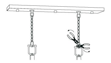
The Mounting Plate is designed to be attached using a center fixture bar and two auxiliary bolts. Attach fixture bar to Center Support Nipple. Secure bolts to structural support rated for load.
