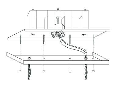
Attach shade by placing over socket. Secure with shade spacer and shade
