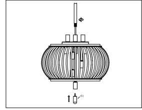
Step.3: Run Stem (D) through Cage (E) and attach Light Cluster (F) to Stem (D). Install G9 LED bulb (G) provided, and carefully lower the cage (E) back over Lamp Cluster (F).
