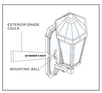
For assemble the MOUNTING BALLS, please note that you are required to apply a small amount of Silicone sealer to the threaded side of the MOUNTING BALLS and then install them onto the MOUNTING SCREWS.
