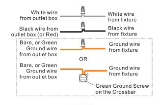
STEP 6 - Install the Fixture Body
