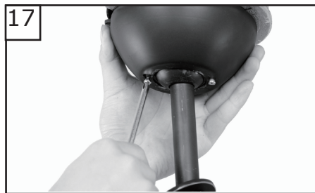
17 Lift canopy up, aligning its keyhole slot with the preassembled screw on mounting bracket and twist till lock. Install the screw removed in step 12. Tighten all screws securely.
