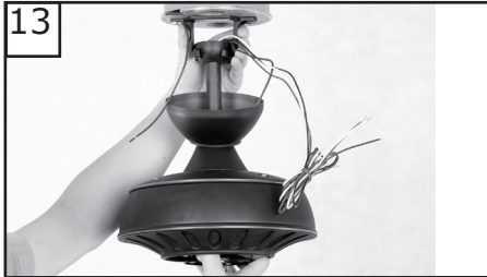
13 Hang assembled fan from the mounting bracket installed to ceiling in previous step. Make sure the fan is hanging straight. Rotate fan until the tab on the Mounting bracket engages the slot on the Downrod Ball. This must be done to prevent the fan body from rotating when the blades are in motion.
