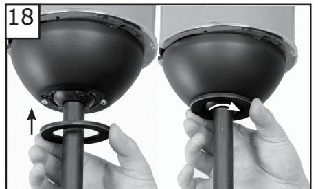
18 Attached canopy bottom cap onto canopy by aligning its notches with the screws on mounting bracket and twist clockwise till tight.
